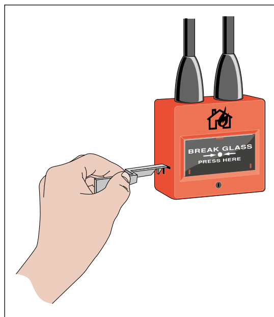
Figure 18: Using a test key
