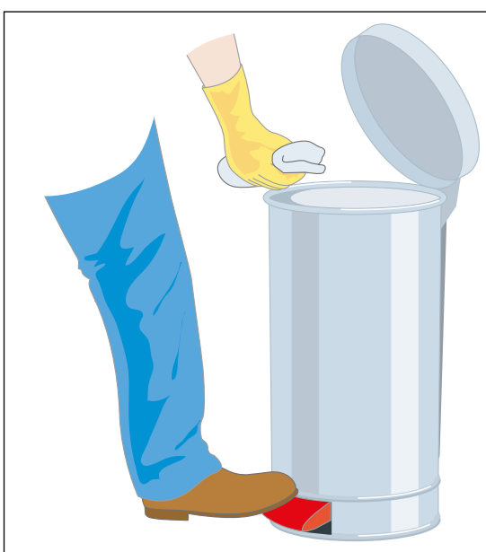
Figure 15: A fire-resisting pedal bin for rags
