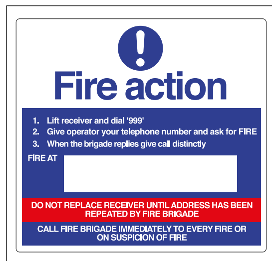
Figure 62: Typical staff fire action notice
